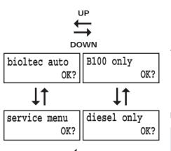
The **bioltec®** system runs in the last selected operating mode until you select another operating mode in the menu and confirm it with the OK key.
