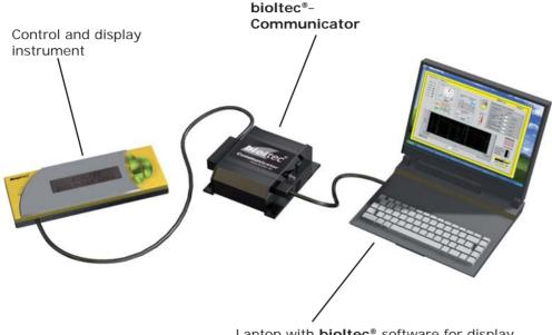
Laptop with **bioltec**® software for display and parameter setting, and for downloading and release changes.
